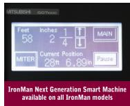
Use the touch screen to automatically control product length, add for miters, if applicable, and keep a total of daily material ran and total footage. Password protected.
